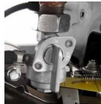
4. If the engine is cold, move the Choke Lever to on position as shown by the arrow.
